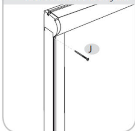
2-B Screw the cassette onto the guides
